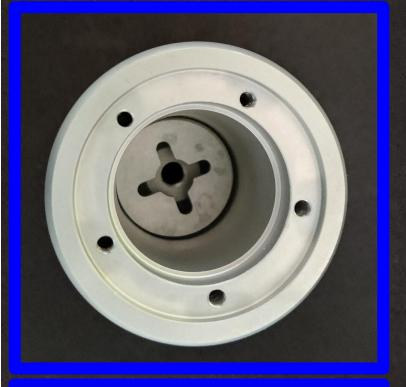
Remove caphead screw with 5mm allen key and seperate two halfs of shifter.
